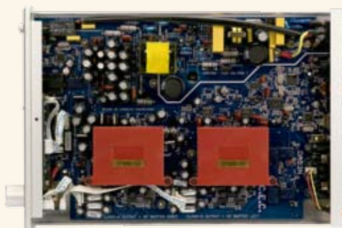
◀ DA53N interior with the red casings for the two LEF amplifier modules visible.
