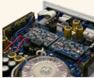
▲ A large 50W toroidal transformer in a compact body. Balanced left/right independent circuitries.
