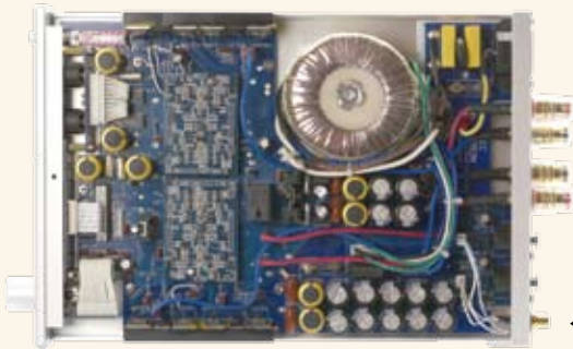
▲ A large 50W toroidal transformer in a compact body. Balanced left/right independent circuitries.
