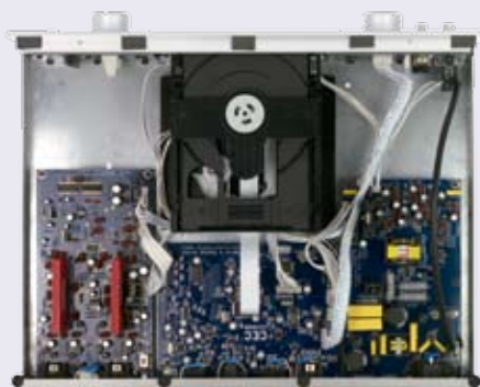
▲ A fully balanced design circuitry with a minimal-length signal path.
