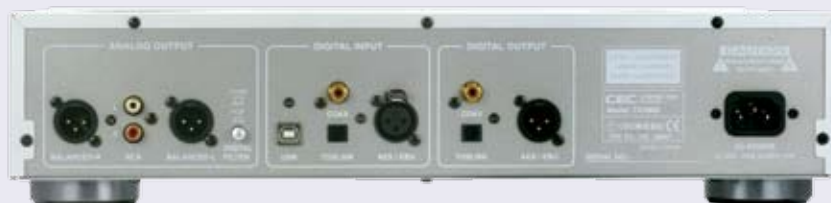
▲ A wide variety of input/output terminals : four different digital input connections (RCA, TOSLINK, AES/EBU, USB) , two different analog output connections (RCA, XLR) and three different digital output connections (AES/EBU, COAXIAL, TOSLINK). The selector switch of the digital filter (FLAT/PULSE) is also on the backpanel.
