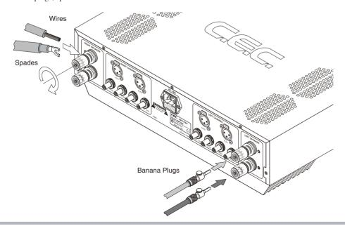
Note: Make sure to turn the AMP6300 off when connecting speaker cables.
