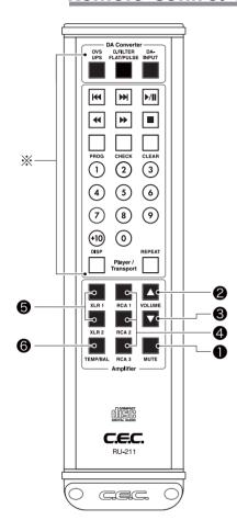
\* The other buttons on the provided remote control unit will work with CEC's line of CD players (such as the CD5300), but are not used for the AMP6300.
