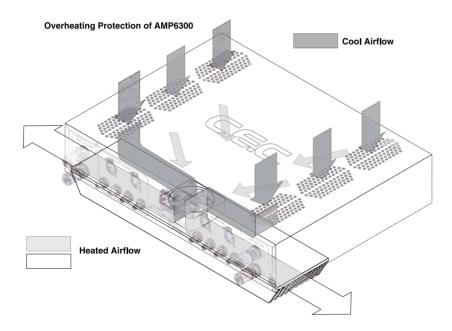
Dusty environments may cause the AMP6300's cooling fan to malfunction. The
