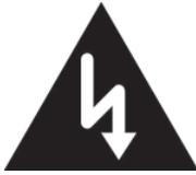
The lighting flash with arrowhead symbol, within an equilateral triangle, is intended to alert the use to potential shock hazards within the product's enclosure.
