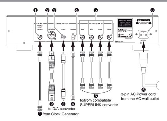
Make a connection before power on, otherwise TL2N may malfunction due to interference when contacting a cable plug to a terminal. Turn off and on again to recover the function.
