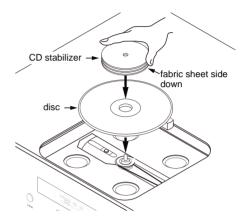
**Important**: Make sure that a disc and the CD stabilizer have been set correctly and laterally before closing the CD door.
